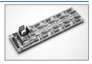
When used for bridge measurements, the EXP-GP allows the bridge completion resistors to be mounted either on or off the board. In addition, two user-installed resistors can be set to form one-half the bridge for all 8 channels. A relay and optional calibration resistor allows a simple shunt calibration.
